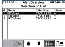
Display of alarm list. Details of each alarm and individual settings is shown.
